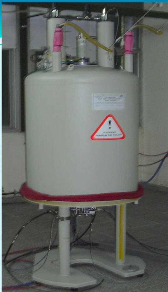
4.7 T superconducting magnet, equivalent to a frequency of 300 MHz for protons.
